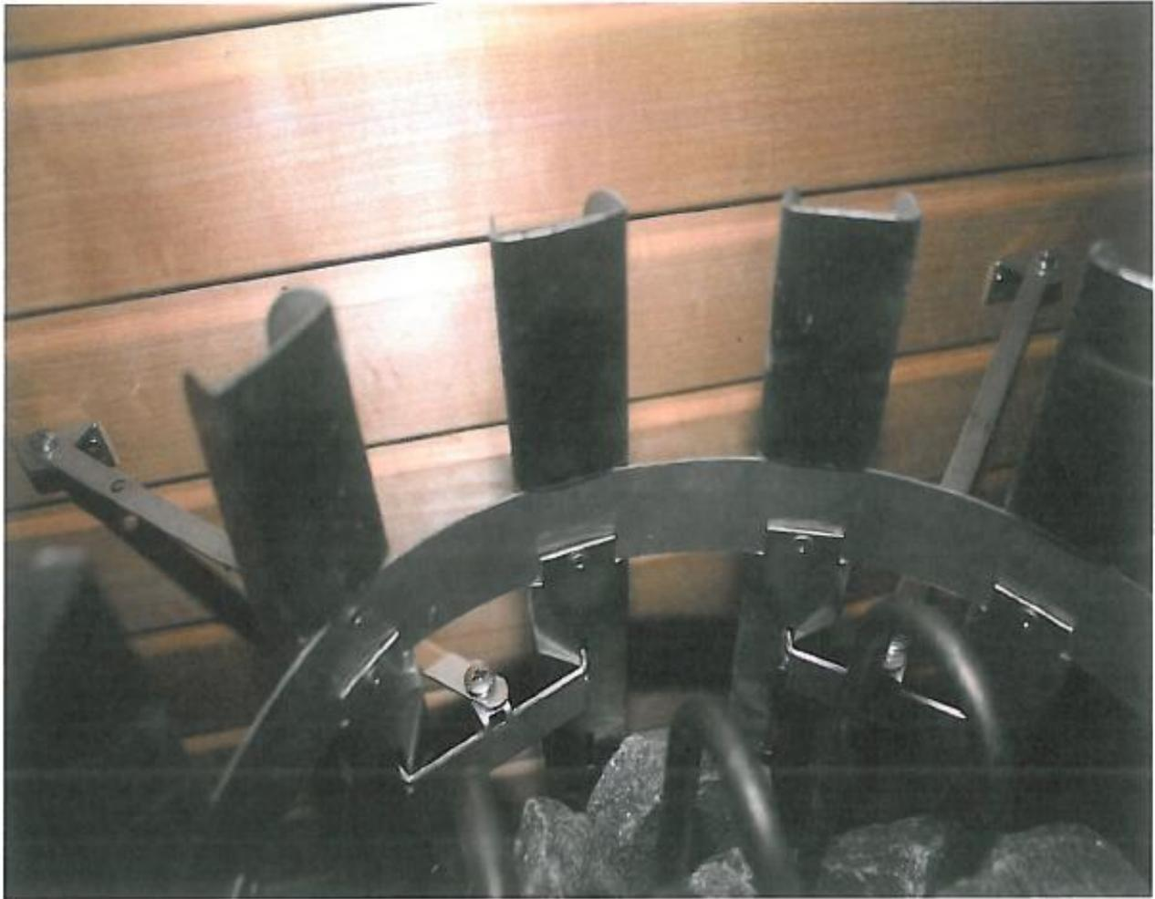
1. Press the supporting iron to be placed within the sauna stove to the bottom of the groove.
